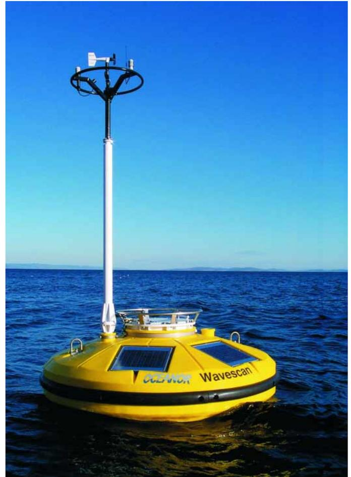
Additionally, the buoy can be equipped with numerous other sensors such as oxygen, hydrocarbon, gamma radiation measurement and an optical sensor for algae detection, to meet the client's specific configuration requirements.
