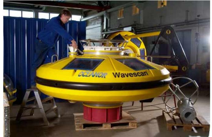
**Fabrication of a Wavescan buoy in Norway**
