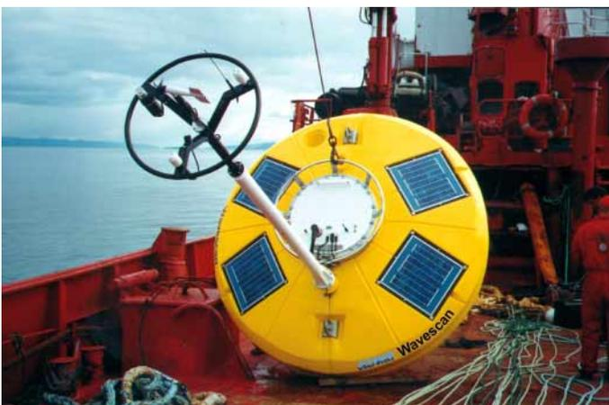
**A Wavescan buoy on board ready for deployment**
